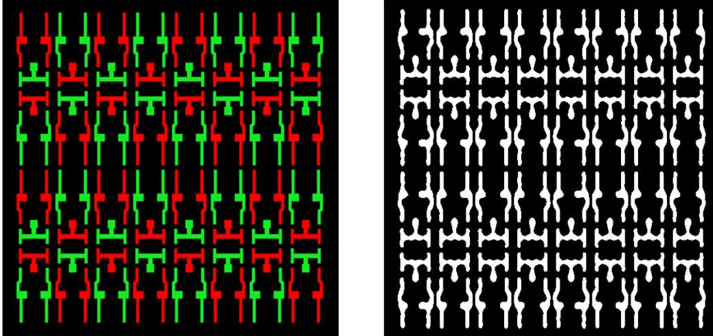
Figure 8. An example of a real IC topology (memory) allows applying “strong” phase-shift technology. Minimal distance between elements is equal to about  $\lambda/2$ , where  $\lambda$  is a reconstructing radiation wavelength. This topology allows bicoloring in such a way that every two elements having a minimal distance between them are colored with different colors.
